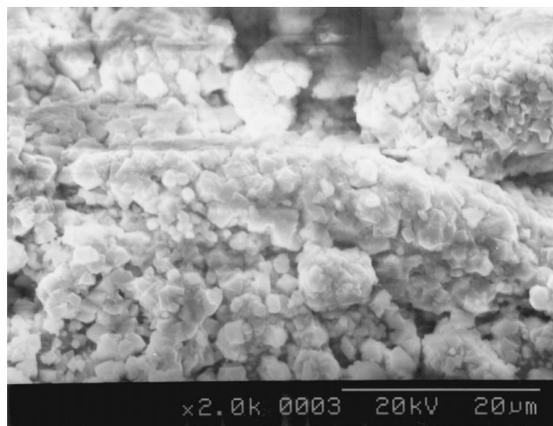
Figure 10 The SEM secondary electron image of surface morphology of the Cu-deposited alumina particle from experiment 16.
